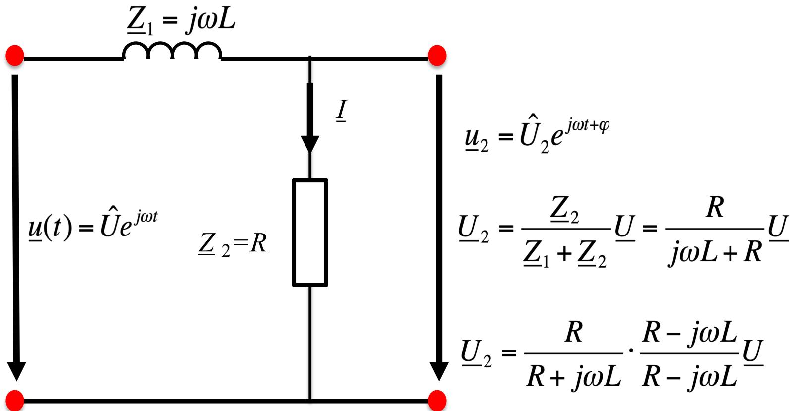
$$\underline{U}_2 = \frac{R^2 - j\omega RL}{R^2 + \omega^2 L^2} \underline{U} \quad \rightarrow \varphi = \arctan\left(\frac{\text{Im}}{\text{Re}}\right) = -\arctan\left(\frac{\omega L}{R}\right)$$
