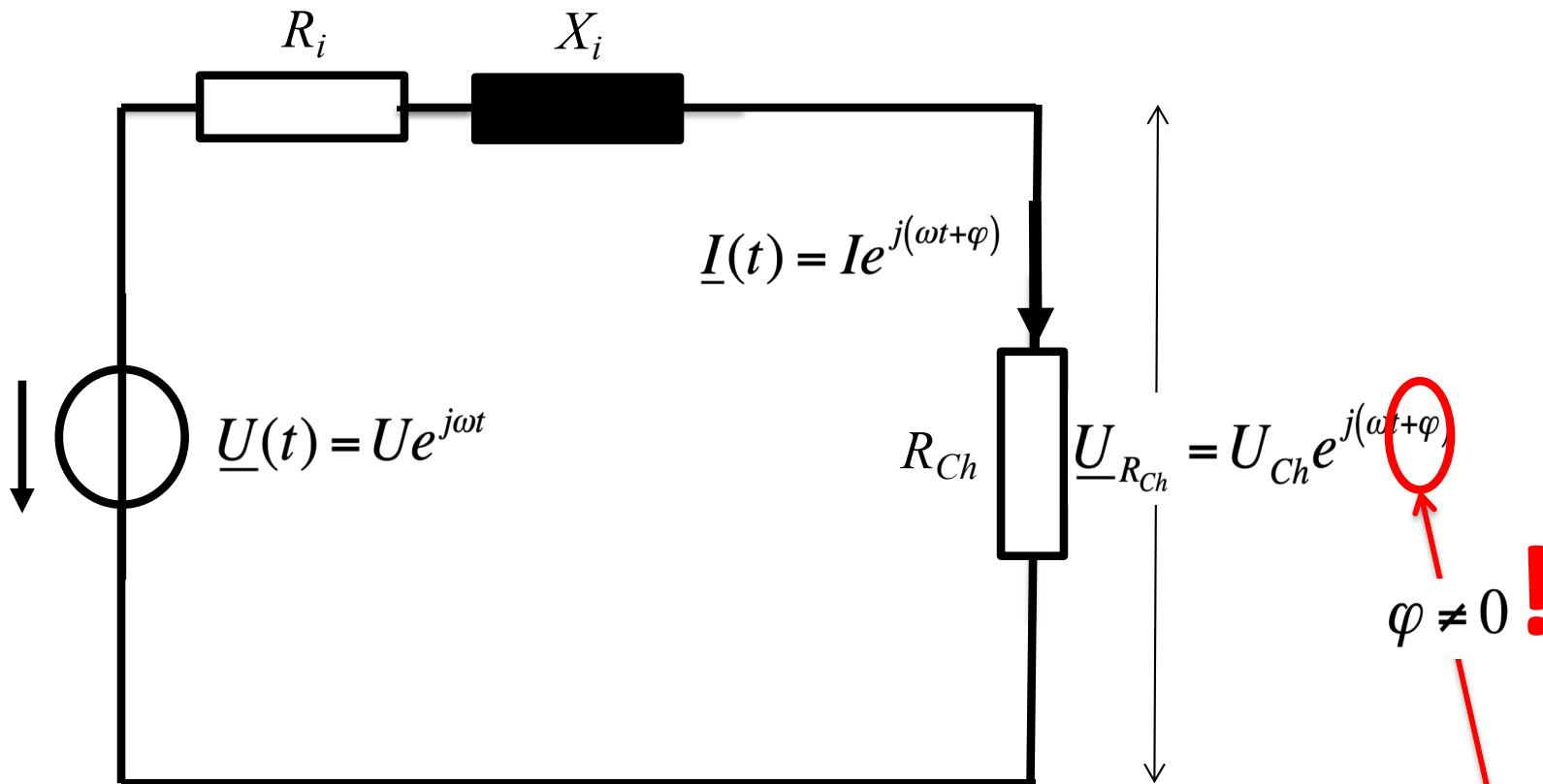
$$\underline{I} = \frac{\underline{U}}{R_i + jX_i + R_{Ch}} \Rightarrow \text{tg}(\varphi) = -\frac{X_i}{R_i + R_{Ch}}$$
