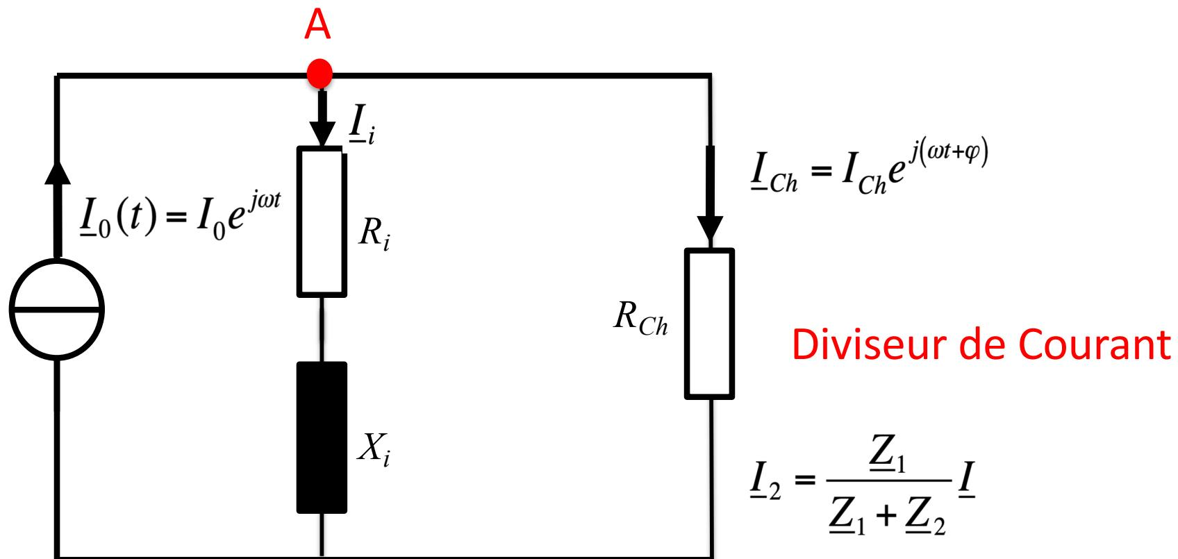
$$\underline{I}_{Ch} = \frac{R_i + jX_i}{R_i + jX_i + R_{Ch}} \underline{I}_0$$
