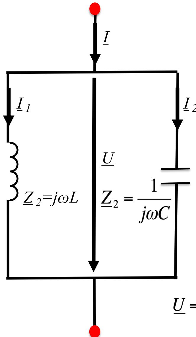
$$Z_{//} = \frac{\underline{Z}_1 \underline{Z}_2}{\underline{Z}_1 + \underline{Z}_2} = \frac{j\omega L}{j\omega L + \frac{1}{j\omega C}}$$
