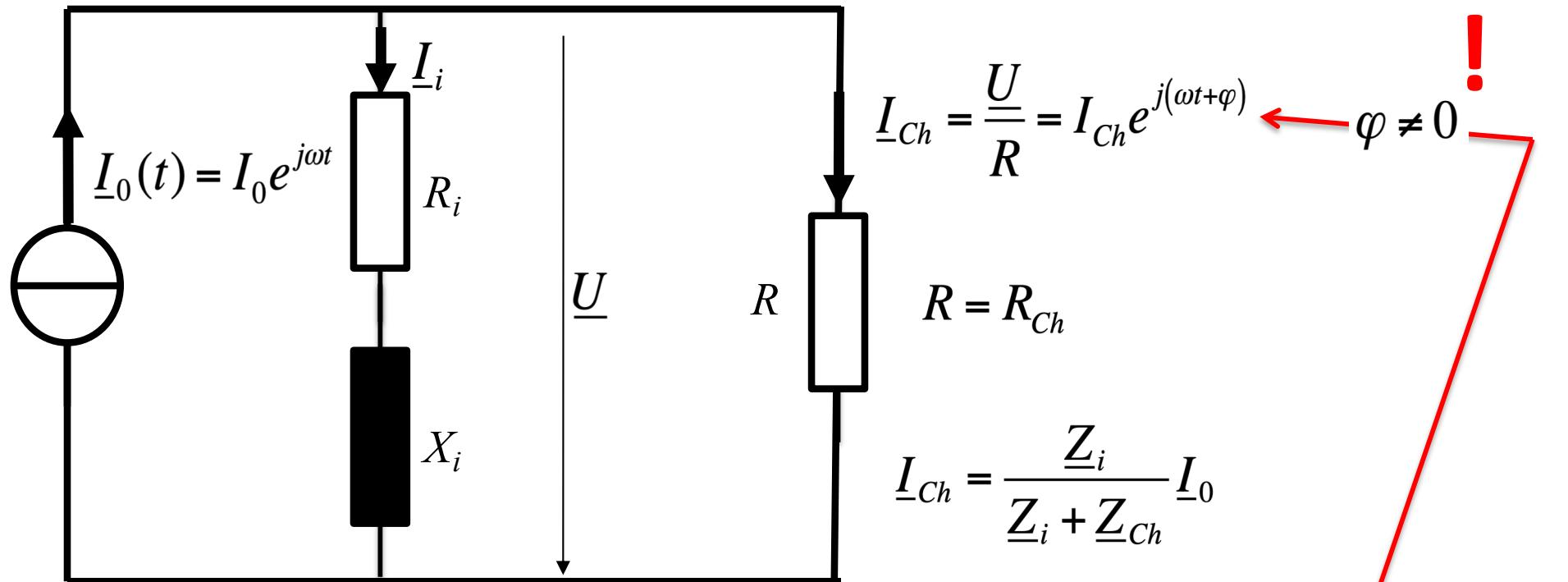
$$\underline{I}_{Ch} = \frac{R_i + jX_i}{R + R_i + jX_i} \underline{I}_0 \cdot \frac{R + R_i - jX_i}{R + R_i - jX_i} = \frac{R_i(R + R_i) + X_i^2}{(R + R_i)^2 + X_i^2} \underline{I}_0 + j \frac{X_i(R + R_i) - R_i X_i}{(R + R_i)^2 + X_i^2} \underline{I}_0$$
