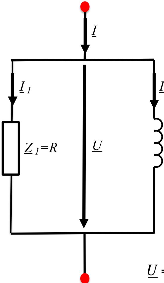
$$\underline{Z}_{//} = \frac{\underline{Z}_1 \underline{Z}_2}{\underline{Z}_1 + \underline{Z}_2} = \frac{j\omega RL}{R + j\omega L}$$
